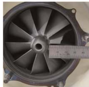
Figure 10: Damaged turbine blade.
