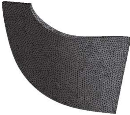
Figure 6. Baseline mesh for FEA analysis.
