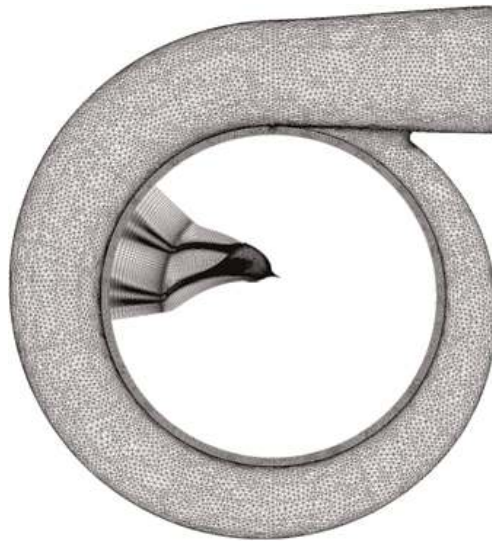
Figure 8. Compressor mesh detail.
