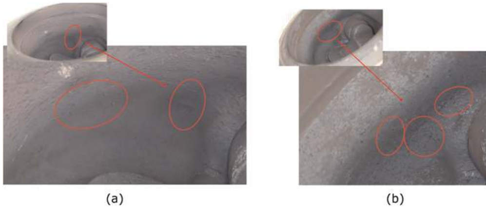
Figure 17. Component level durability test for 150hrs at location 3 (a) Conventional steel (b) Nitrogen steel.
