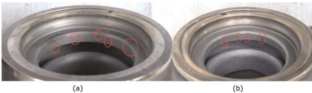
Figure 16. Component level durability test for 150hrs at location 2 (a) Conventional steel (b) Nitrogen steel.
