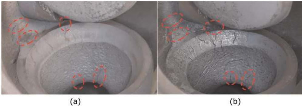
Figure 15. Component level durability test for 150hrs at location 1 (a) Conventional steel (b) Nitrogen steel.
