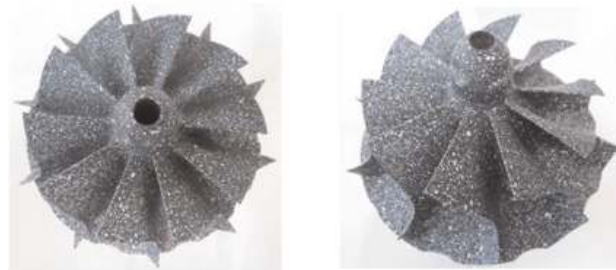
Figure 11. Random speckle pattern painted on the turbine impeller.
