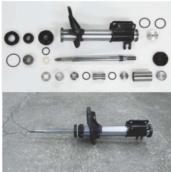
Fig. 3. Photograph of the manufactured MR damper
