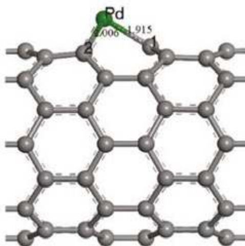
Figure 19. Geometric structures of Pd-doped SWCNTs after optimization. The structural parameters are shown as Å.
