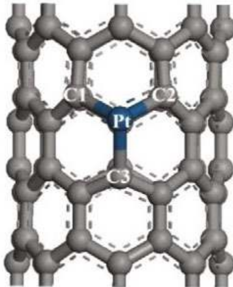
Figure 35. Geometric structures of Pt-doped SWCNTs after optimization. The structural parameters are shown as Å.
