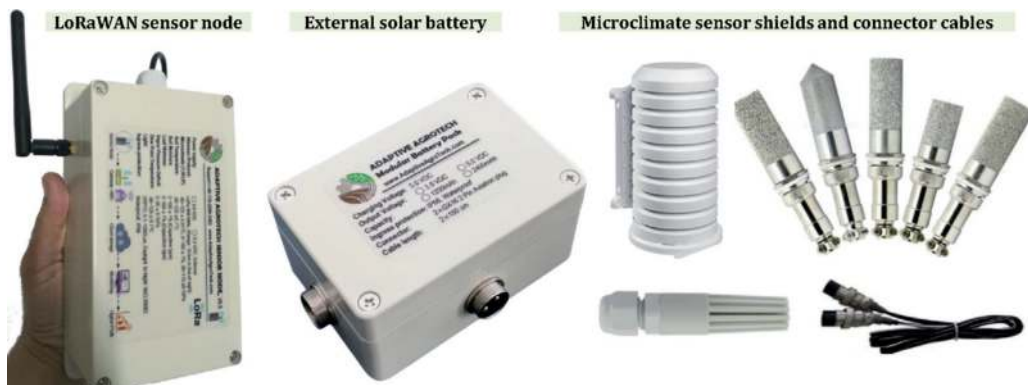
Figure 2. A LoRaWAN wireless sensor node with an external solar-charged battery and different sensor shields used in real-time monitoring of greenhouse microclimate parameters. Images by courtesy of Adaptive AgroTech.
