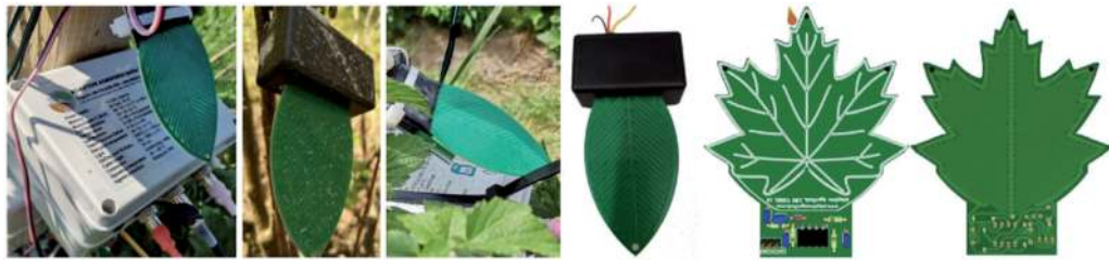
Figure 6. ADP-AgroTech leaf wetness sensor (model ADP-LWS2020) with different leaf shapes based on capacitive method for determining leaf surface moisture and greenhouse condensation. Images by courtesy of Adaptive AgroTech
