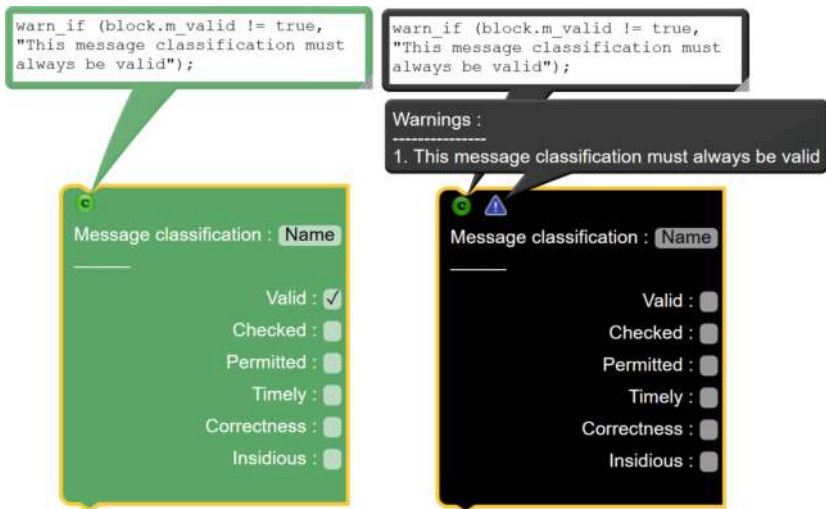
Fig. 21. An example of a constraint where the member variable m_valid is checked
