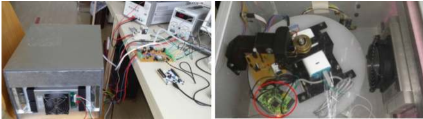
Fig. 3. Experimental chamber for obtaining training data for the compensation model. On the right the prototype of the CDC module has been highlighted with a red circle and is mounted on the rotating plate.
