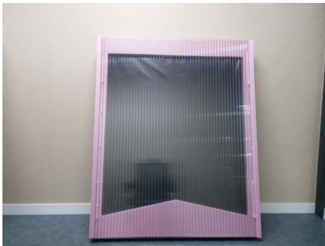
Figure 9. One square metre effective area MES prototype with 10 layers, whose weight is 15 kg.
