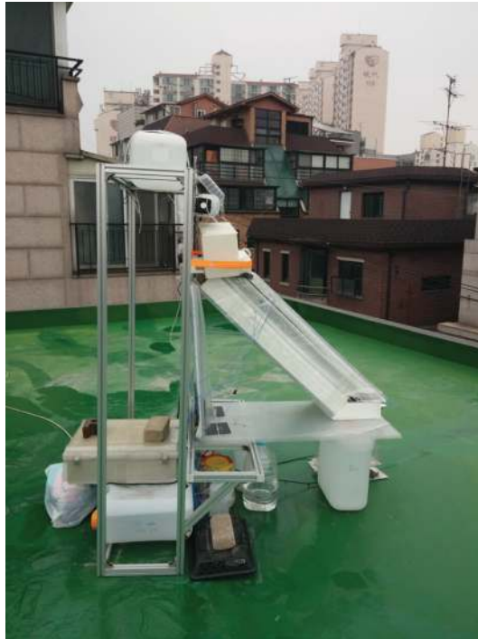
Figure 8. MES system installed tilted 45°.
