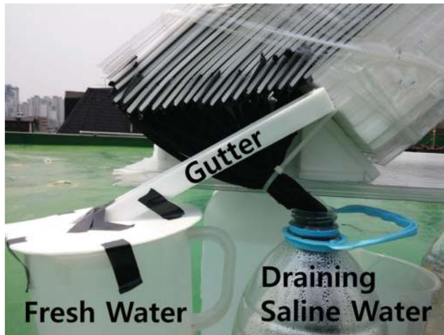
Figure 11. Collecting fresh water from each layer by a gutter.
