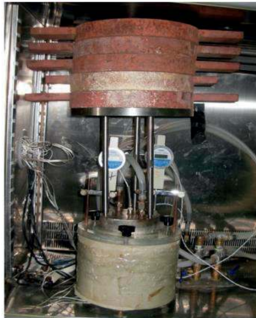
Figure 2. Loading apparatus used for the frost heave test.
