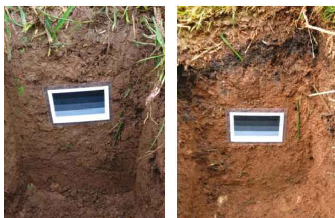
Figure 1. Two examples of topsoil profile imagery captured using the smartphone camera. The colour correction card in each image is approximately 10 cm long and 6 cm wide.
