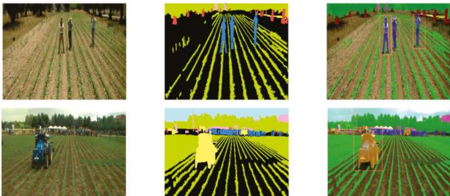
Figure 18. Peoples and a vehicle identified as obstacles in the working environment.
