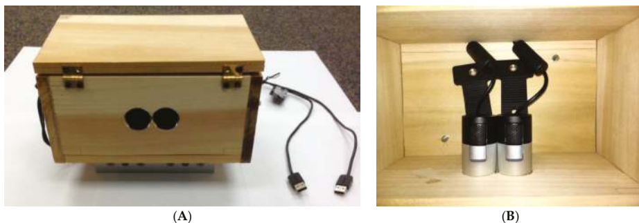
Figure 1. Stereo cameras which are used to acquire images: (A) whole view; (B) inside view.
