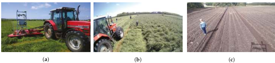
Figure 2. Images from experiments and recordings. (a) The sensor kit mounted on a mower; (b) An example image from the recordings in grass; (c) An example image from the recordings in row crops.
