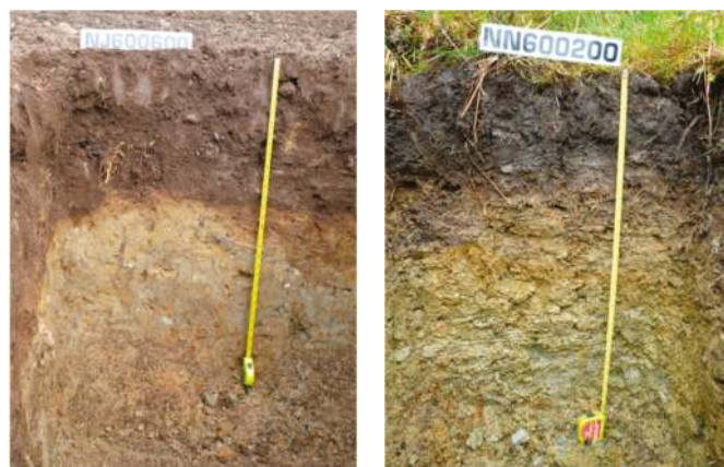
Figure 2. Two examples of soil profile imagery captured during the NSIS2 field campaign. A tape measure was placed against each profile to provide scale. In each image, the tape length is 75 cm. Photographs credited to John Bell and Willie Towers.
