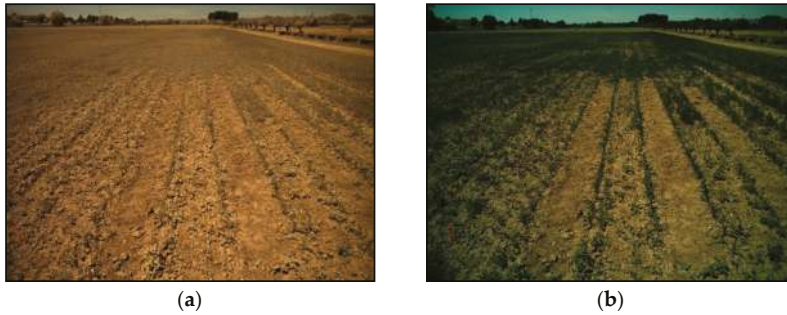
Figure 2. Effect of the UV/IR cutting filtering: (a) without filter; (b) with filter.
