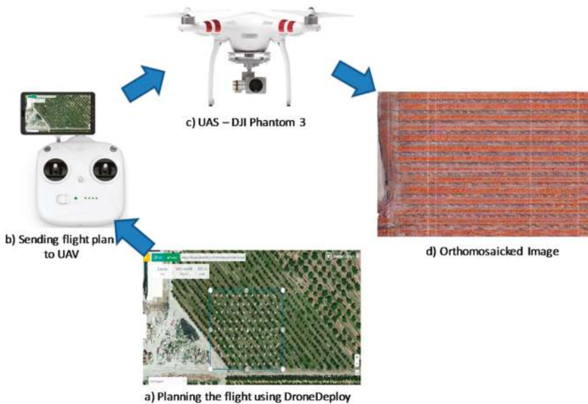
Figure 3. Operation of UAS using DroneDeploy. (a) Planning the flight using DroneDeploy; (b) Sending flight plan to UAV; (c) UAS – DJI Phantom 3; (d) Orthomosaicked image.
