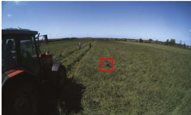
Figure 7. Detections in grass mowing case. Notice that people are not detected.
