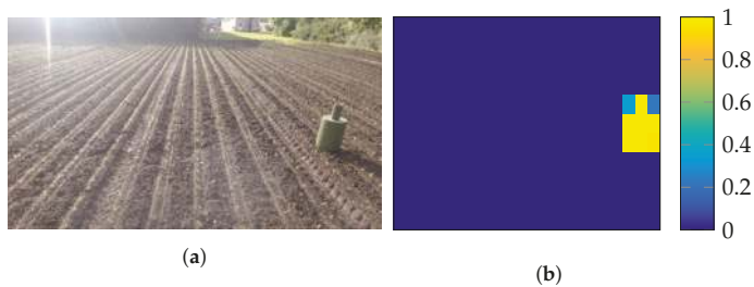
Figure 4. Illustration of ISO obstacle and resulting heatmap. (a) RGB image from the row crop field; (b) Resulting heatmap.
