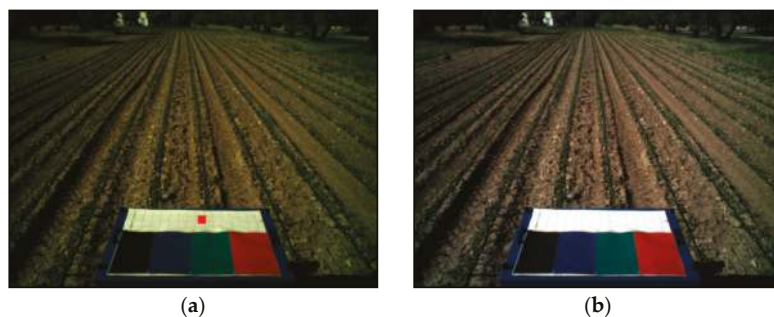
Figure 4. White balance: (a) original image; (b) corrected image.
