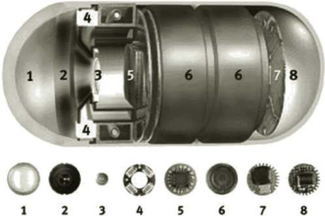
FIGURE 11.2 M2A capsule endoscopy: (1) optical dome, (2) lens holder, (3) lens, (4) illuminating sources, (5) CMOS imager, (6) battery, (7) transmitter, and (8) antenna.
