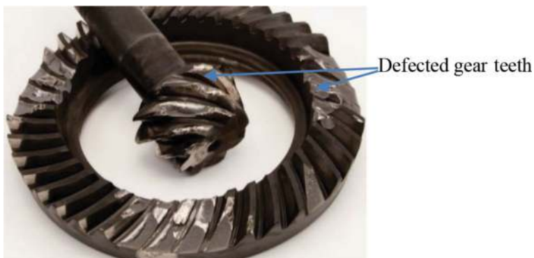
Figure 8. Example of the gear defects [30].
