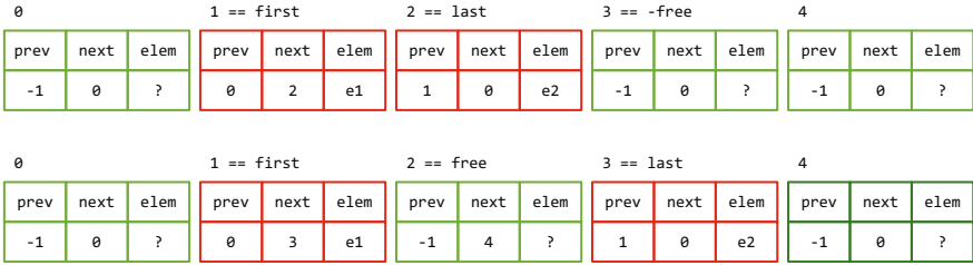
Fig. 2. Two doubly linked lists of capacity 4 and length 2
