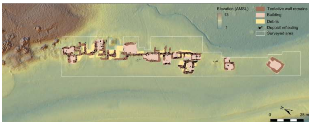
FIGURE 7.6 Plan and digital terrain model of the trading site Maríuhöfn (or Búðasandur) in Hvalfjörður, Iceland, after a geophysical survey carried out in 2015. Image by Ronny Weßling, Joris Coolen, Natascha Mehler © HaNoA project.
