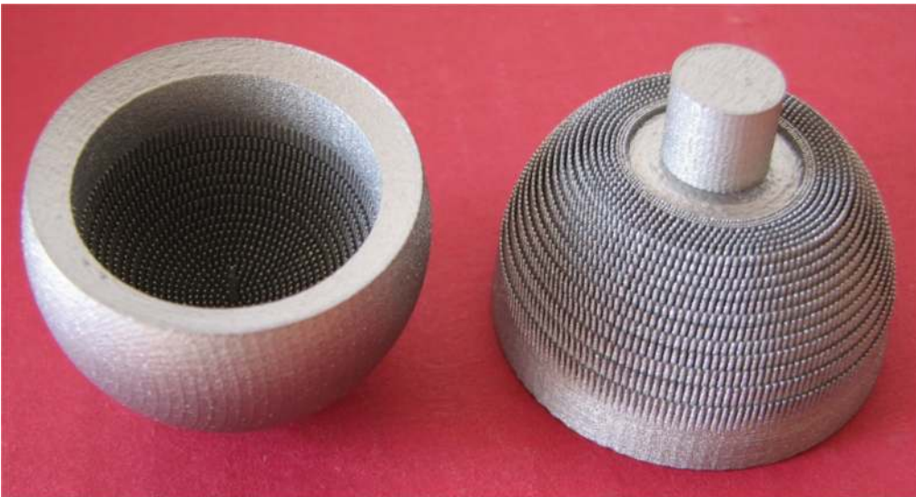
FIGURE 3.30 Prototypes produced in SLM technology required further precise processing (turning, grinding, polishing, lapping of the cooperating articulate surface of hip joint endoprotheses); visible technological handles allow precise surface finishing.
