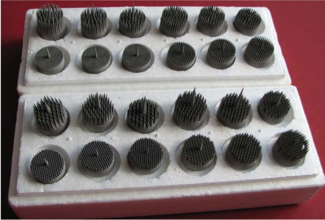
FIGURE 3.26 A set of 24 preprototypes of the MSC-Scaffold produced by SLM technology.
