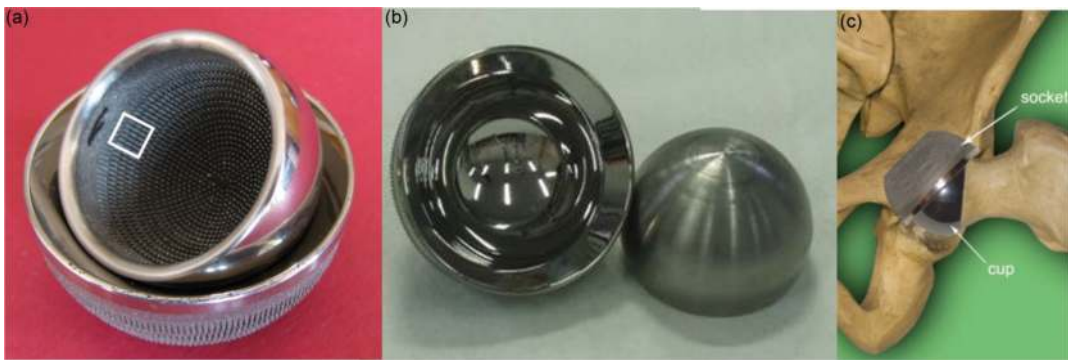
FIGURE 3.31 A prototype of a resurfacing endoprosthesis of the hip joint with the MSC-Scaffold: (a) and (b) after grinding and polishing the articulate surface, (c) illustratively in the hip joint.
