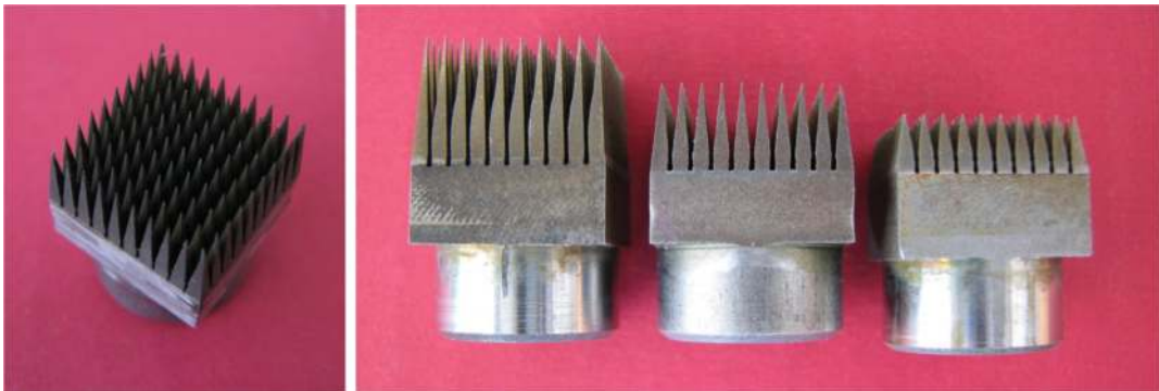
FIGURE 3.18 Trial geometric structures of the MSC-Scaffold of the prototype resurfacing endoprosthesis of the hip joint manufactured with the use of the wire-cut EDM method with three different heights of the spikes.
