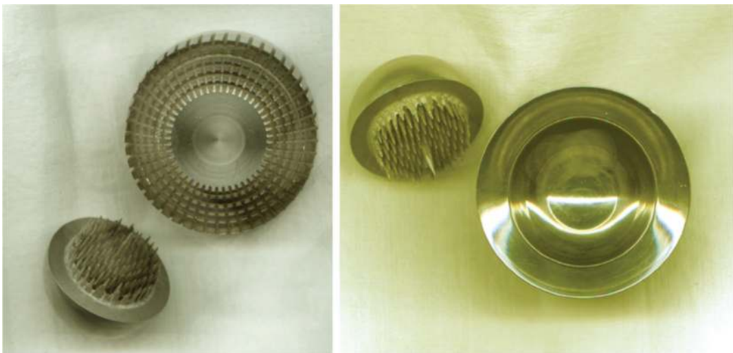
FIGURE 3.15 An early (unsuccessful) demonstration prototype of a hip joint resurfacing endoprosthesis, made for chrome steel using the die-sinking EDM.
