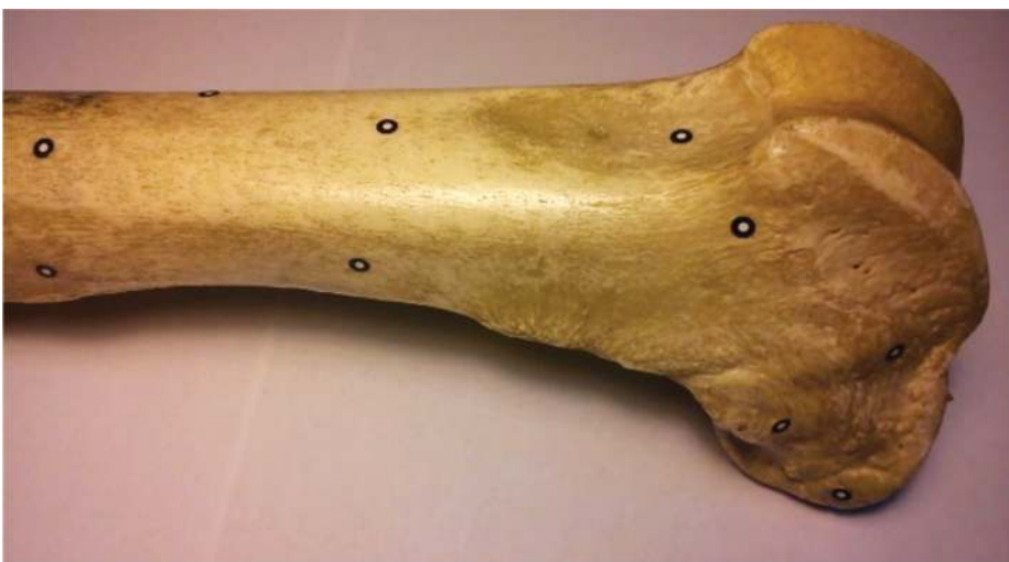
FIGURE 3.42 Swine femur prepared for optical scanning.
