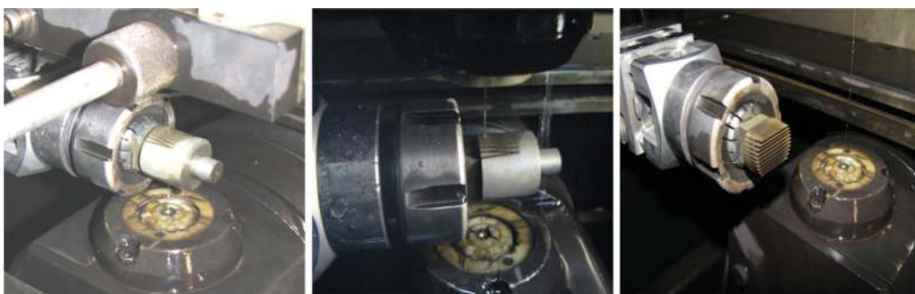
FIGURE 3.17 Wire-cut EDM of a trial geometric structure of the MSC-Scaffold; the illustrations present the cutting trajectory.
