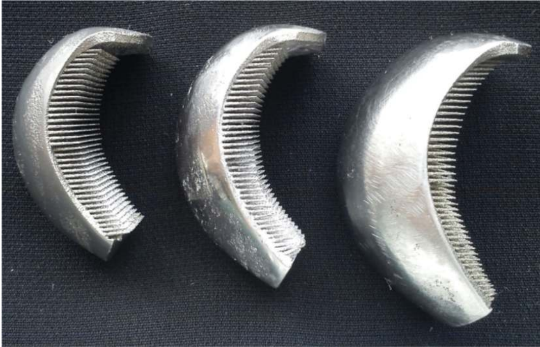
FIGURE 3.51 A range of sizes designed (CAD) and manufactured in the SLM technology of working prototype of partial resurfacing knee arthroplasty endoprosthesis with the MSC-Scaffold.
