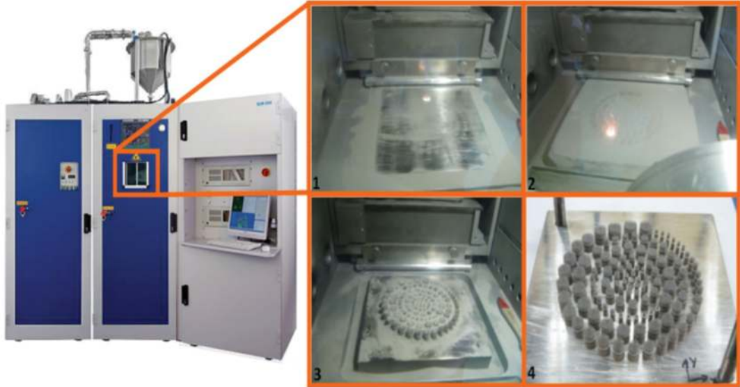
FIGURE 3.35 The main steps of the additive manufacturing process of the preprototypes of the MSC-Scaffold with the SLM machine (ReaLizer SLM 250, MTT Technologies): (1) selective laser melting of one of the first powder layers, (2) selective laser melting of one of the last powder layers, (3) cleaning of the produced nonmelted powder preprototypes, (4) as-manufactured preprototypes printed on board.
