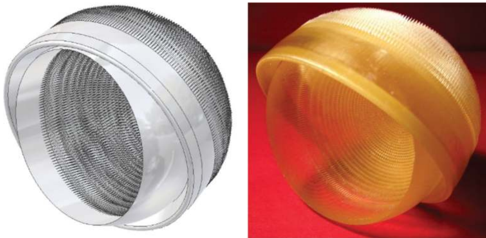
FIGURE 3.23 The solid CAD model and the resulting demonstration prototype of a resurfacing arthroplasty endoprosthesis with the MSC-Scaffold.
