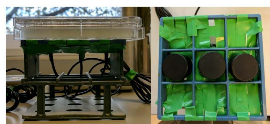
Figure 2. Acoustic parameters (left) and experimental set-up for sonication of MSSA-'N' biofilms (right). The sonicating probes were in direct contact with the 24-well polystyrene plate using ultrasound gel. Each well housed three alginate beads with nutrient broth +/- gentamicin during treatment.
