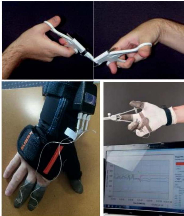
Figure 23. Contact pressure measurement, generated during the use of laparoscopic instrumental.
