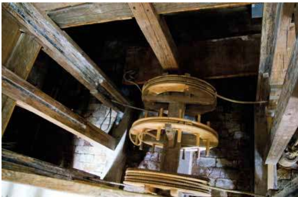
5.3 Table hoist, c. 18 th century, Confidence Room, Chinese Pavilion, Royal Palace, Stockholm. © Fabian Persson.
