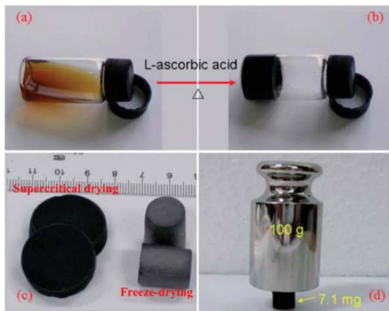
Figure 1. Digital photos of the aqueous suspension of graphene oxide (a), the graphene hydrogel in a vial (b), the graphene aerogels obtained by supercritical CO 2 drying and freeze-drying (c), and a graphene aerogel supporting a counterpoise (d) [17].
