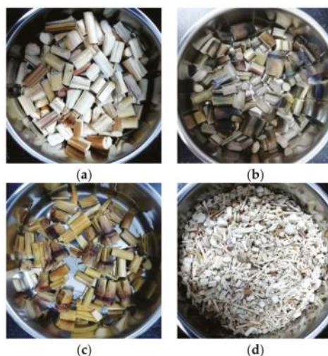
Figure 1. (a) Non-treated corn straw; (b) corn straw treated with acid (solid-liquid ratio 1:20, soaked in 20% HCl for 24 h, washed, and then dried to constant weight); (c) corn straw treated with alkali (solid-liquid ratio 1:30, soaked in 1% NaOH for 24 h, washed, and then dried to constant weight); and (d) comminuted corn straw.
