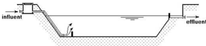
Figure 4.6. Schematic representation of an anaerobic pond
