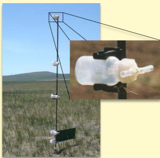
▲ Field Setup: Collection bottles at different vertical heights
