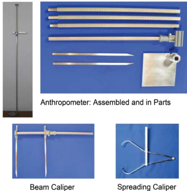
Figure 4.12: Examples of equipment for anthropometric measurements: anthropometer (top) and calipers (bottom). Figures from Gordon et al. 2014 p. 11.
