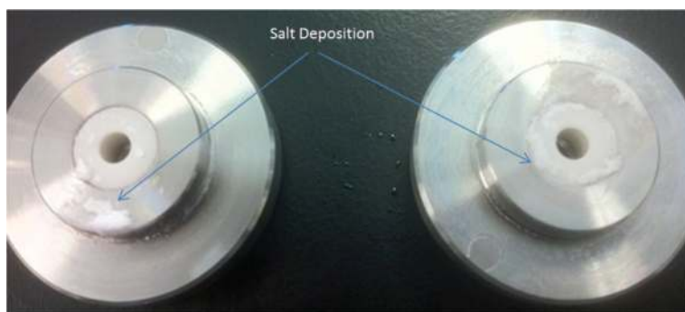
Figure 36. Salt depositions at screws of the column.
