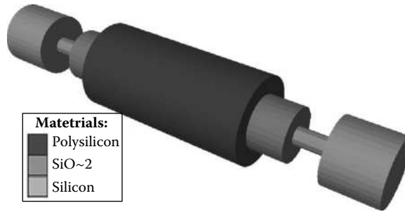
FIGURE 6.34 Simulated schematic structure of the Si-nanowire.
