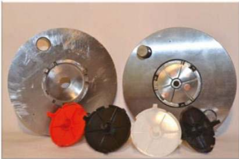
Figure 17. Injected plastic materials obtained at Plastor SA Oradea using the injection moulding tools made by SLM.
