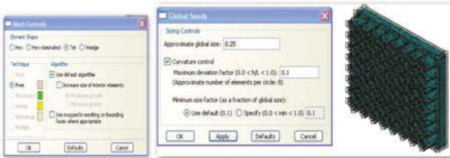
Figure 21. Element-type control and mesh-size control defined for the FEA.
