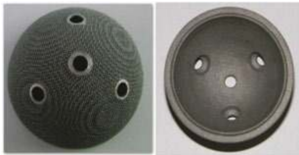
Figure 25. Customized medical implant manufactured from Ti6Al4V material using the SLM 250 HL equipment.
