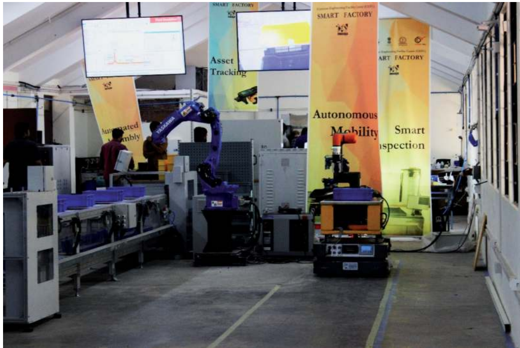
Figure 5. Autonomous mobile vehicle/Hanhwa Cobot system collaborating with robotic arm for material handling process.
