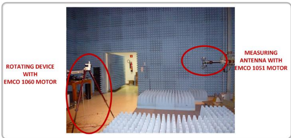
Figure 3. Measuring antenna and positioning devices to obtain the radiation pattern inside the anechoic chamber.
