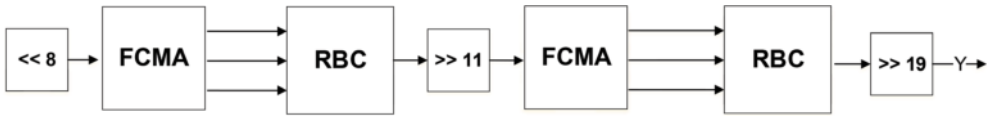
Figure 7. The block diagram of two-level RNS-based DWT design, and FCMA represents FIR-filtering process in RNS.
