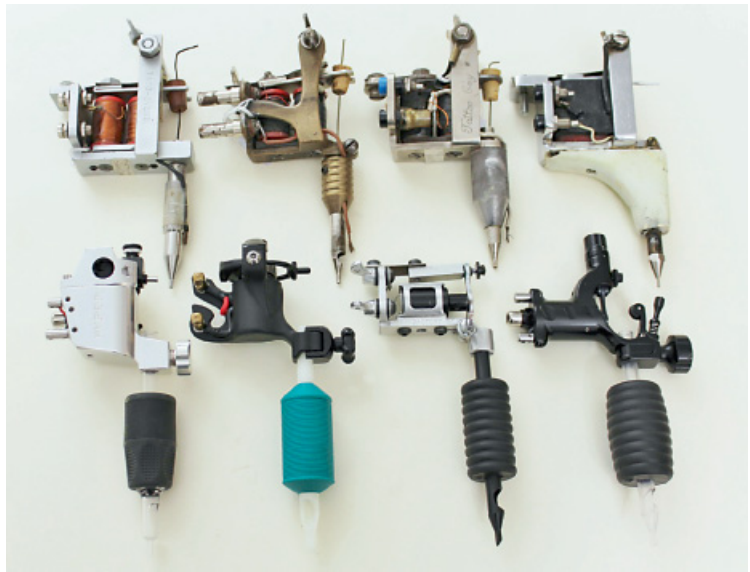
Fig. 1. This photo shows two types of tattoo machines. Old coil machines with fixed tubes and needles are shown in the upper row. This type is still used widely today. The bottom row shows different types of rotary machines with disposable grips. The main difference lies in the weight, materials and possibility of changing tubes and needles, a need that former times did not recognise.
