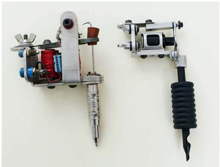
Fig. 2. The machine on the left is an old coil machine from around 1980, one of the first homemade machines I ever used. It has a non-disposable grip. A small, very light rotary machine from 2012 is shown next to it for comparison. It has a disposable plastic grip. Compared to the almost soundless and vibration-free rotary machine, the old machine is very noisy and vibrates violently. This is something that can be felt in the fingers after many years of working as a tattoo artist. The old machines weighed up to 400 g; the rotary machine on the right weighs 80 g.
