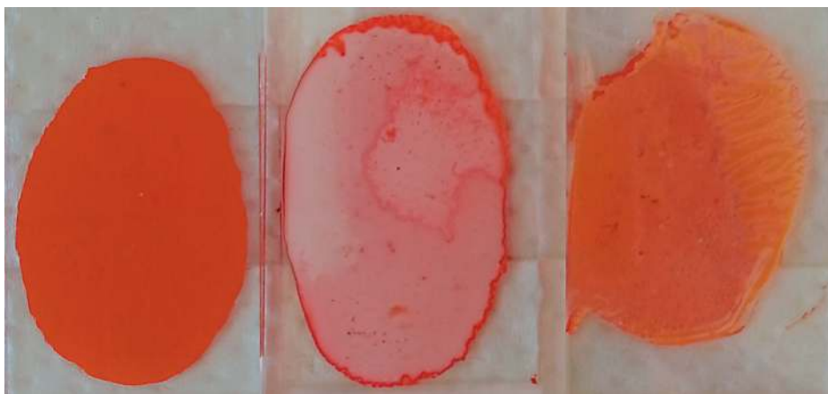
Fig. 1. Orange tattoo ink containing C.I. 21110 and titanium dioxide. From left to right: dark control sample, sample irradiated for 7 days with artificial sunlight, and sample irradiated for 7 days with visible (VIS) light only.
