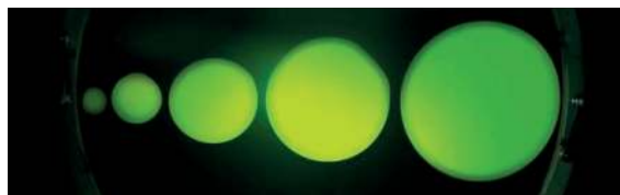
Figure 7. Roundness of holes produced by AWJ.
