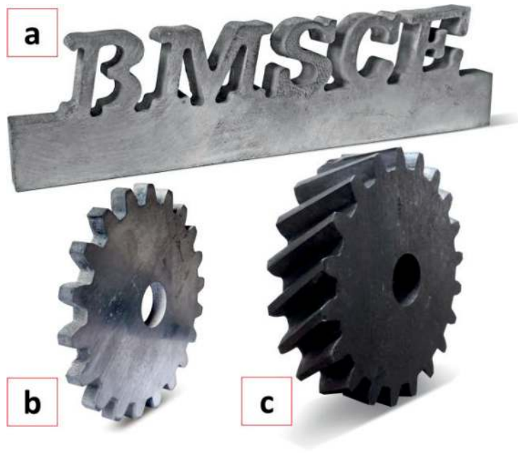
Figure 11. Profile of helical gear produced by AWJ (a) logo in AM60 Mg alloy, (b) spur gear profile in AM60 Mg alloy, and (c) cast iron helical gear profile.
