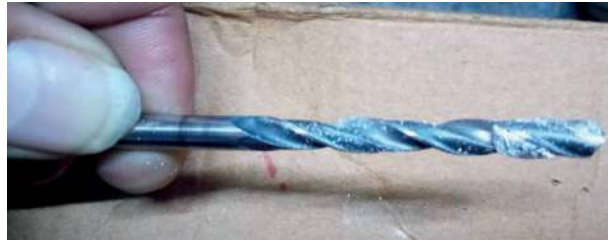
Figure 9. Adhesion of material to the drill bit.
