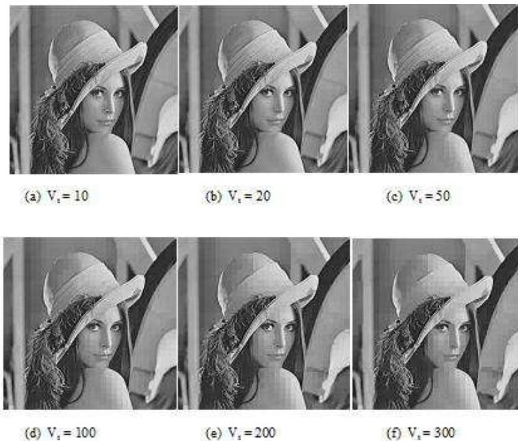
Fig. 1. Reconstructed Lena images with compressed 16*16 blocks with different threshold variances V_t .
