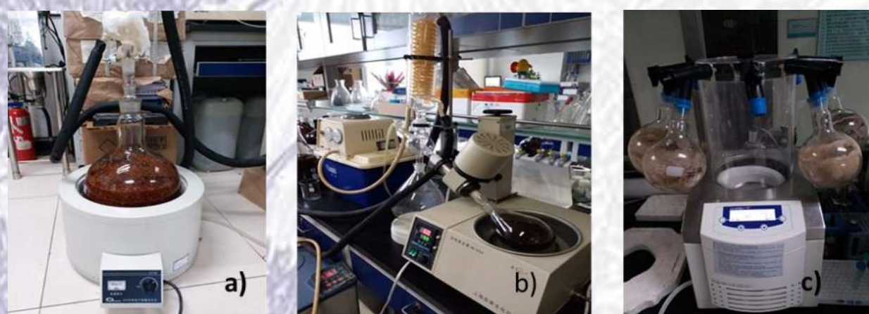
Figure 1. Preparation of the herbal compound JT2016 at the Health-Cultivation Laboratory, Beijing University of Chinese Medicine (a: extraction, b: concentration, c: freeze drying.)
