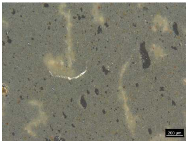
Figure 7.41 The presence of a hair-like material in Fabric type A in XP (JF001) (Photo by Miki)
