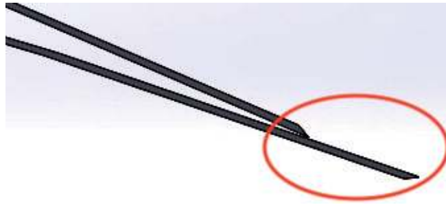
Figure 4. Trailing edge diagonal cut treatment for simplified meshing.
