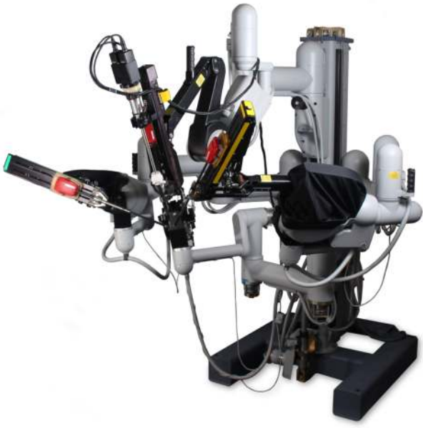
Fig. 1. The da Vinci surgery robot as it sits in the laboratory at Aalborg University. One arm is partially disassembled for easy access to the actuators and sensors.
