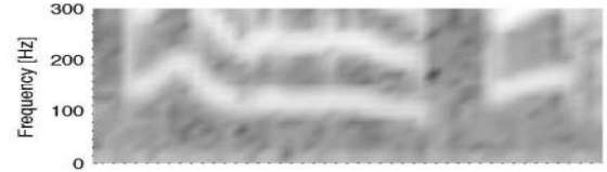
(a) Spectrogram of a speech segment. Note that y-axis is limited to the frequency range containing pitch.
