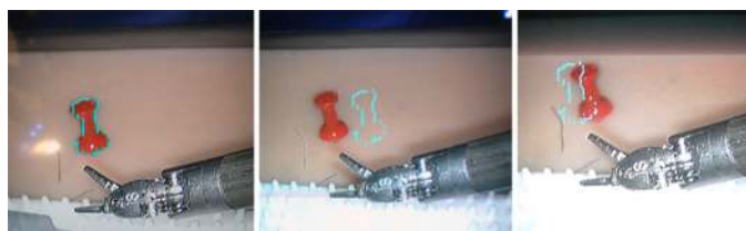
Fig. 2. Telestration. Left: drawing around a pen on the touch screen. Center: the drawing as displayed in the surgeon console’s left display. Right: the drawing in the right display. The drawing gets offset for both eyes, making it appear at a different depth than the background. For some users this creates double vision and thus makes precise pointing impossible.
