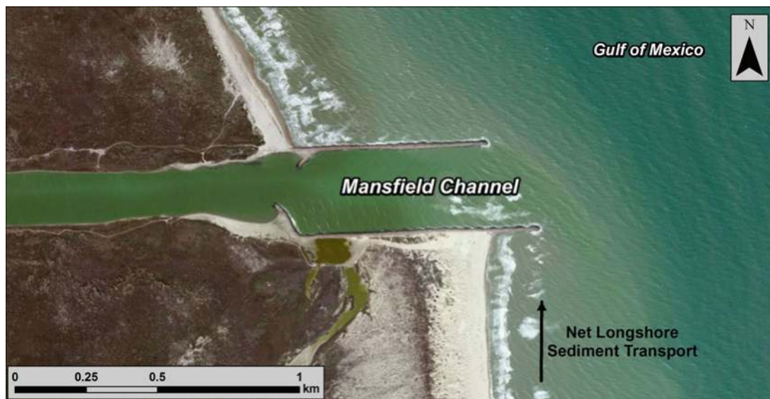
Figure 6.56. Shoreline offset at Mansfield Channel jetties illustrating net longshore transport to the north along South Padre Island, Texas. Image credit: ArcGIS World Imagery.
