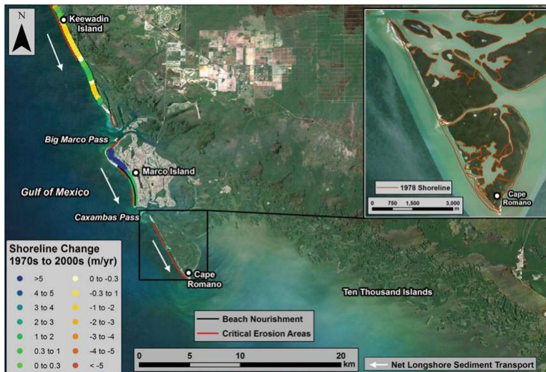
Figure 6.34. Shoreline change from Keewaydin Island to Cape Romano. Most critically eroding shorelines occur in the Cape Romano area at rates of about 5 m/year. Sources: Shoreline change data, Absalonsen and Dean (2010); Cape Romano shoreline position (1978), NOAA (2013a); beach nourishment locations, Miller et al. (2004), FDEP (2008); critical erosion areas, FDEP (2012a). Image credit: Microsoft Bing Maps Aerial.
