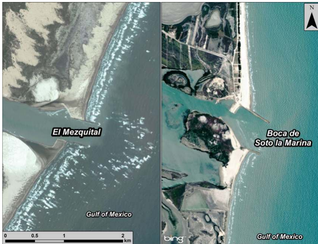
Figure 6.57. Shoreline offset at the El Mezquital and Boca de Soto la Marina entrances along the Tamaulipas Laguna Madre coast illustrating net longshore transport to the south. Image credit: Microsoft Bing Maps Aerial.
