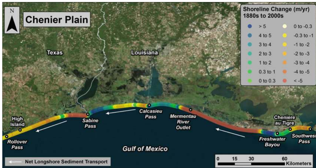
Figure 6.52. Historical shoreline change trends for the Mississippi-Atchafalaya River Chenier Plain coast. Shoreline change data from Martinez et al. (2009) and Paine et al. (2011). White arrows show the direction of net littoral sand transport. Image credit: Microsoft Bing Maps Aerial.
