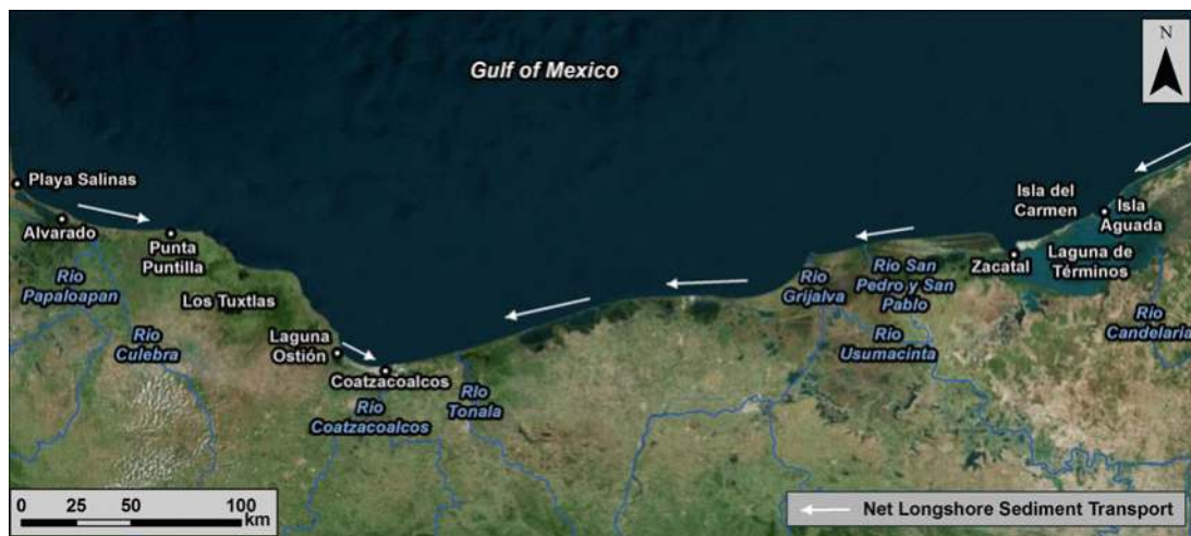
Figure 6.60. Tabascan Neritic shoreline between Playa Salinas and Isla Aguada illustrating variability in the net longshore transport system. White arrows show the direction of net littoral sand transport. Image credit: Microsoft Bing Maps Aerial.
