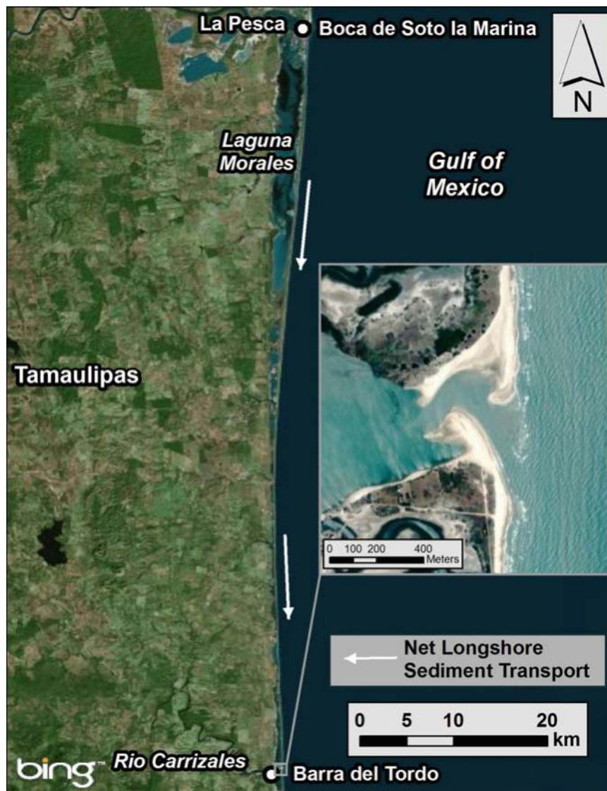
Figure 6.58. North-south shoreline between Boca de Soto la Marina and Barra del Tordo illustrating bi-directional transport at Rio Carrizales in an overall net south-directed longshore transport system. White arrows show the direction of net littoral sand transport. Image credit: Microsoft Bing Maps Aerial.
