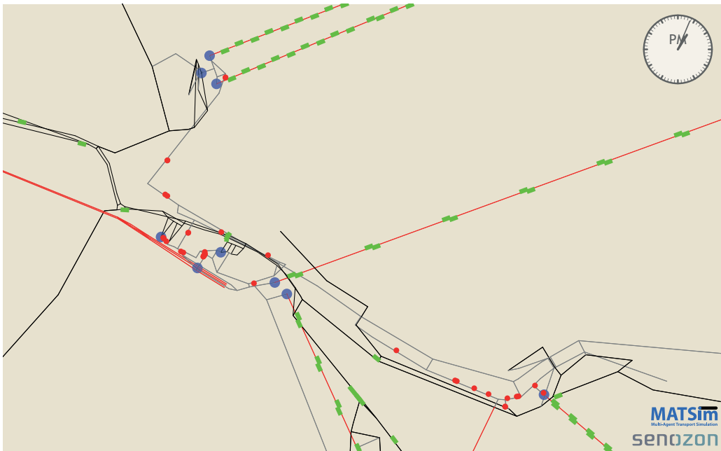
Figure 88.2: Simulated pedestrians (red circles) at Krasnaya Polyana hub. Transit vehicles (incl. cable cars) shown as green boxes, transit stops as blue circles.
