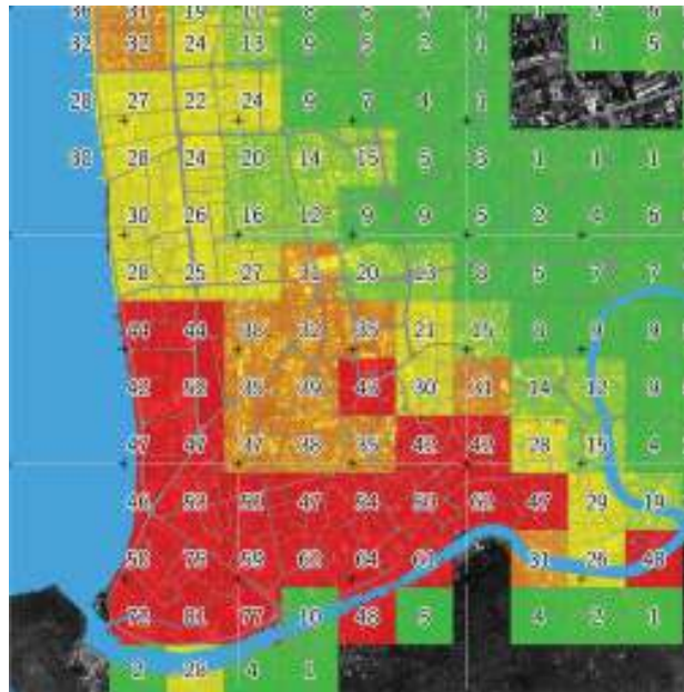
Figure 76.1: Evacuation time analysis for downtown Padang. Numbers showing average evacuation time in minutes, which are also indicated by the colors green, yellow, red.
