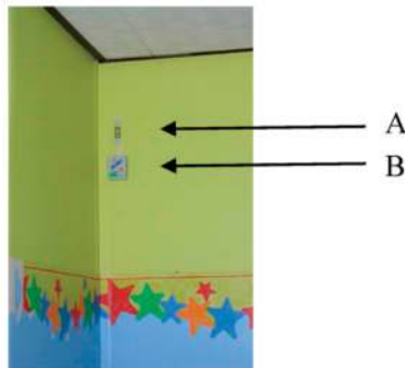
Figure 1. Typical sensor locations on the inside of the external wall in an index child's bedroom ( A : fungal detector, B : temperature and relative humidity logger).
