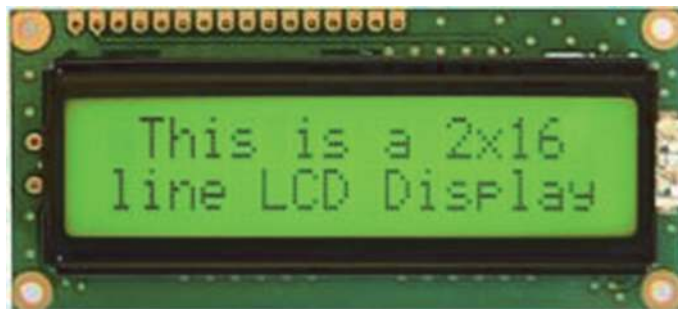
Figure 1. 2 \times 16 LCD physical picture [5].
