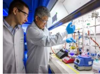
Vacuum gas manifold
