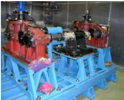
Fig. 3. Gear fatigue test rig overall view
