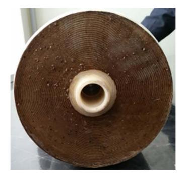
Figure 3.4 Bio-fouled spiral-wound RO membrane.
