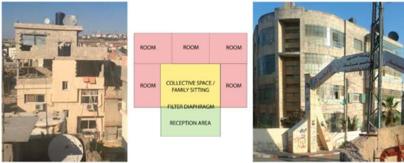
Figure 2. Refugees building homes. A family house built in the camp (left) and outside the camp (right). Although the aesthetics of the respective facades are radically different, their floor plans follow the same scheme developing around a central collective space (in yellow). Areas in red identify the most private parts of the house, accessible exclusively by the resident family (bedrooms, bathrooms, kitchen). Source: the author.
