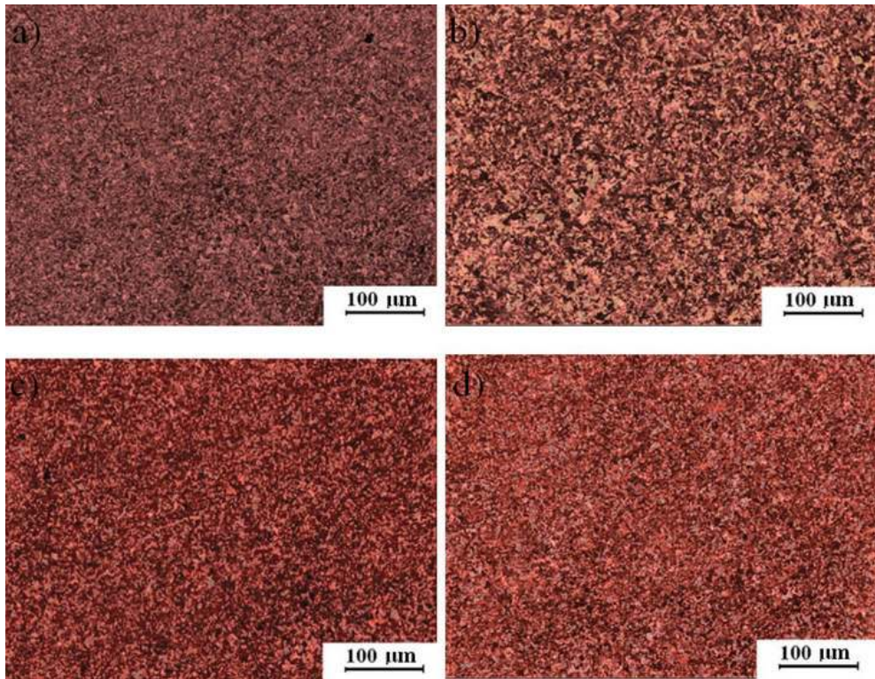
Figure 13. Optical photographs of the microstructure of the copper after three passes of "rolling-pressing" process: (a) initial microstructure, (b) annealing, (c) quenching, and (d) normalizing.
