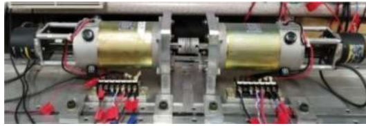
Figure 4. Photograph of the experimental two-mass resonance model.
