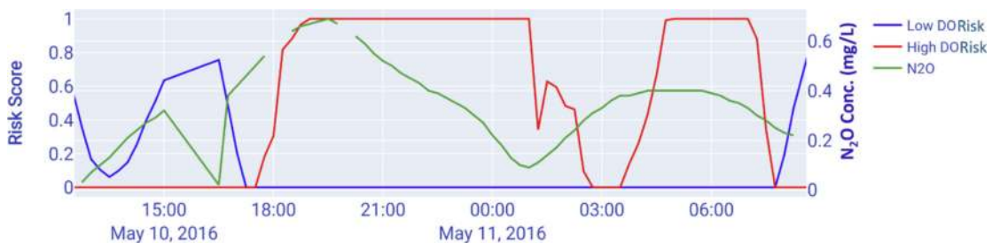
Figure 10.1 N 2 O risk and aqueous N 2 O measurement results for Eindhoven WWTP (NL).
