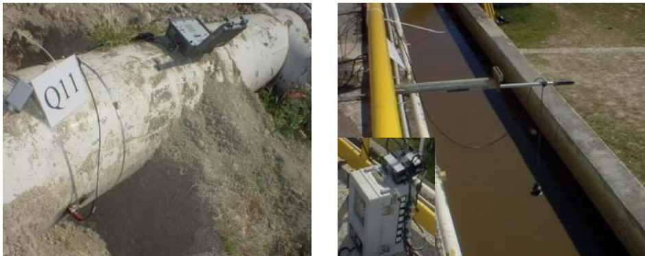
Figure 12.3 Flow measurements in closed full tubes (left) and in an open canal (right).
