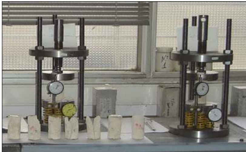
Figure 9. The collected intact calcarenitic rock specimens from Mustafa Kamel Necropolis site under creep testing devices.
