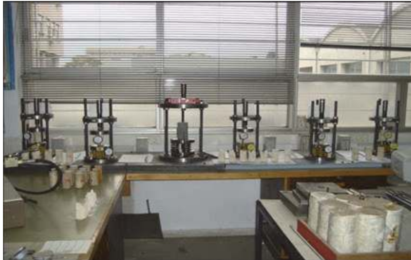
Figure 6. Rock creep testing devices. Samples are 90–105 mm high, 42–44 mm 2 diameters. Two displacement sensors were used during each test.
