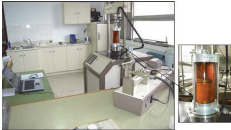
Figure 18. Triaxial creep test device, with constant axial load under confining pressure. Triaxial creep test device. The cylindrical specimen placed inside (GDS) cell is loaded vertically using the compression machine.
