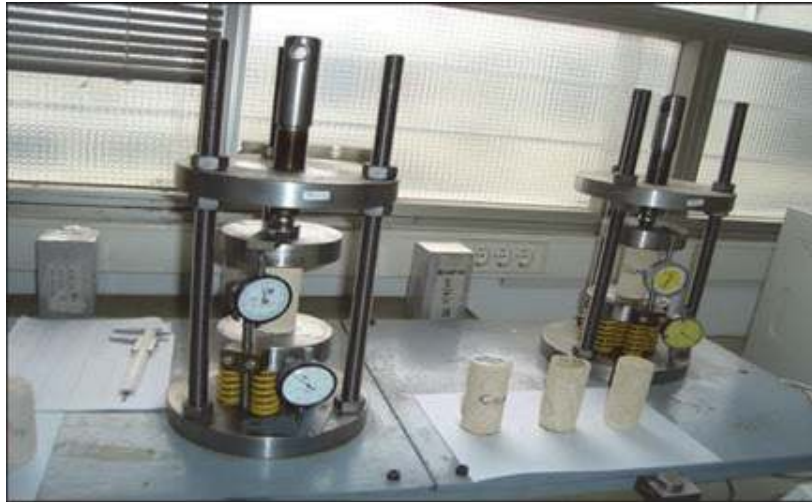
Figure 8. The collected sandy oolitic limestone specimens from the catacombs of Kom El-Shoqafa site under creep testing devices.
