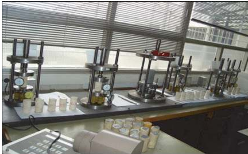
Figure 7. The collected intact sandy oolitic limestone specimens from El-Shatby Necropolis site under creep testing devices.
