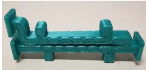
Figure 3. Printed model of a Ka-band diplexer with two band-pass filters with elliptical response.
