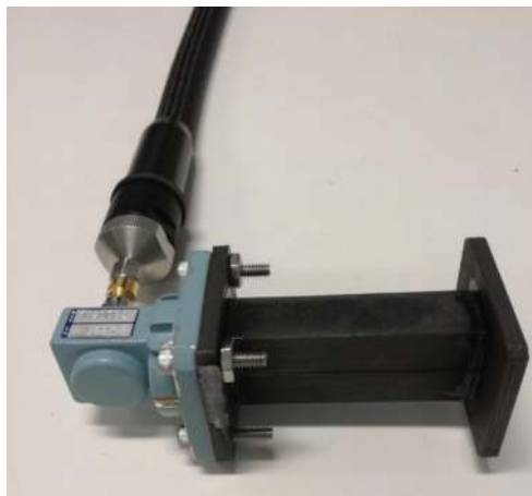
Figure 11. Measurement setup of the waveguide load.
