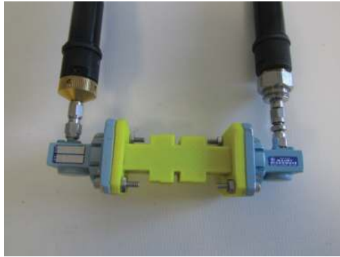
Figure 15. Measurement setup for the low-pass filter connected to the VNA.
