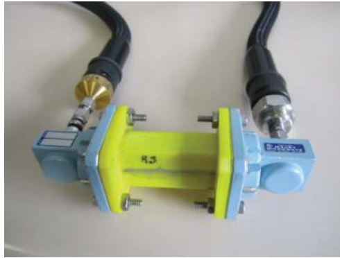
Figure 5. 3D printed WR75 waveguide section ready to be measured.
