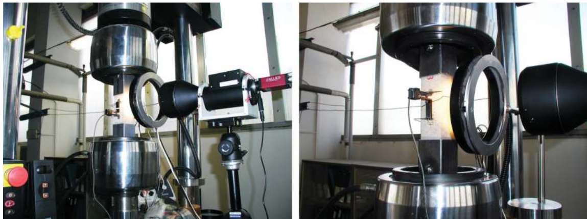
Figure 5. Arrangement of pure tension tests on the stone specimens (photo by M. Šperl).
