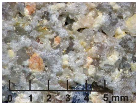
Figure 3. Macro photo of the Božanov sandstone (arkose) structure (photo J. Frankl).
