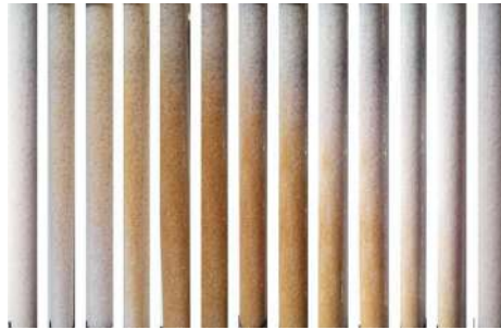
Figure 10. Saturation and regeneration processes evolution observed in the photocatalytic filter (PR2).
