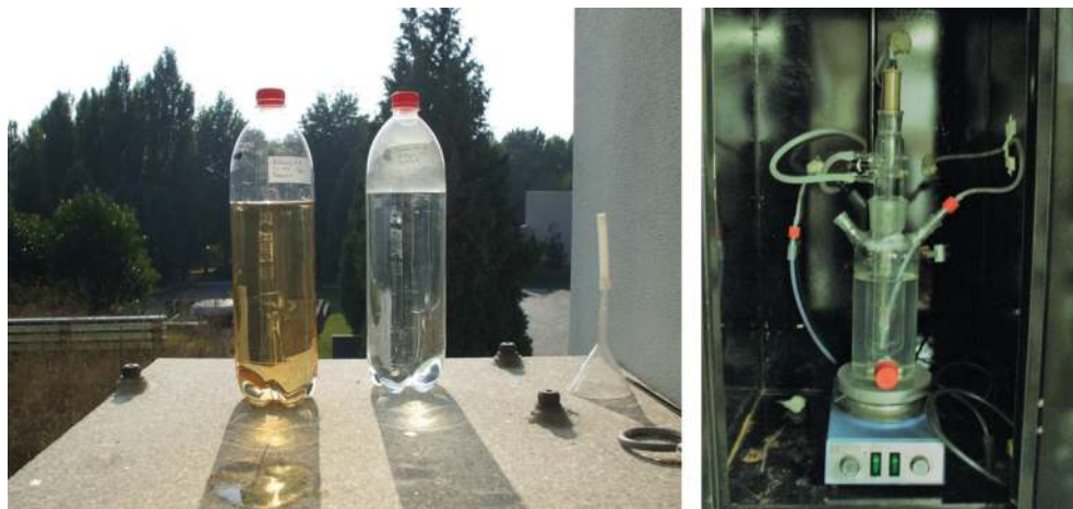
Figure 2. UV radiation sources used in OTC degradation experiments: solar (polyester bottles); UV reactor Heraeus Noblelight .
